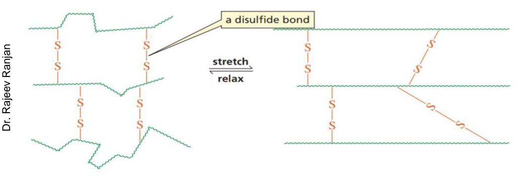
The physical properties of rubber can be controlled by regulating the amount of sulfur used in the vulcanization process. Rubber made with 1–3% sulfur is soft and stretchy and is used to make rubber bands. Rubber made with 3–10% sulfur is more rigid and is used in the manufacture of tires. Goodyear's name can be found on many tires sold today. The story of rubber is an example of a scientist taking a natural material and finding ways to improve its useful properties.
