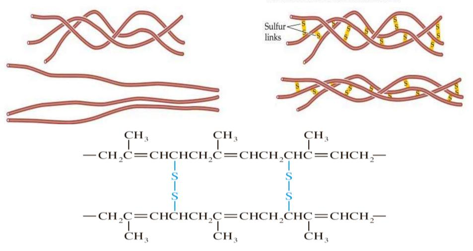
In the segment of vulcanized rubber shown below, the chains of polymerized isoprene are cross-linked by sulfur-sulfur bonds, giving the polymer more
