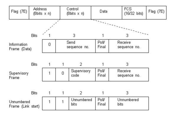
The HDLC frame begins and ends the error checking procedure with **01111110** in binary.
